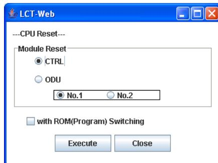
6 Select on control button “CTRL” for IDU or “ODU” or “No. 1 or No. 2” (in 1+1 ODU only), and click “Execute” button in CPU Reset tab,
